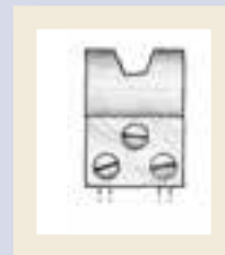
Figure 1C. V-notch four-way tension adjustable trigger
