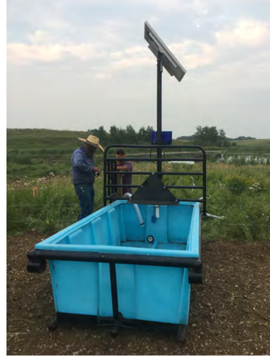
A solar-powered watering system for cattle that are fenced away from water sources. The system is attached to a trailer so that it can easily be moved around the property as livestock are rotated.
