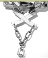
Figure WC19c. Compound levers
