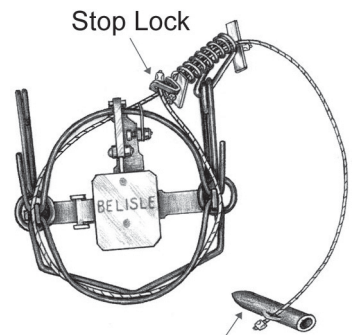
Spring-activated Cable Device
