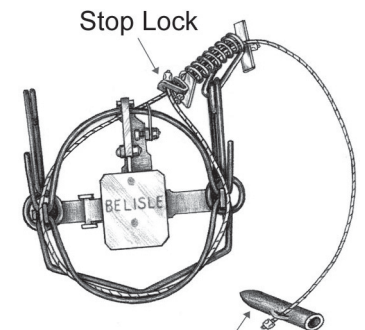
Coil-Spring Activated Cable Device
